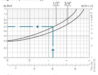
Reference values: Upstream pressure = 8 bar Downstream pressure = 3 bar
